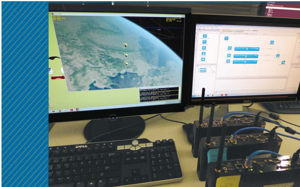
FIGURE 4. The runtime platform's deployment. The simulator image (on the left) shows three satellites, whereas the other display (on the right) shows the deployment model of the experiment.
