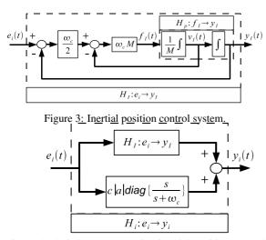
Figure 4: Strictly output passive inertial position control system.
