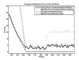
Figure 13: Average and maximum errors of UAVs' positions (time-varving delay and nacket loss case).
