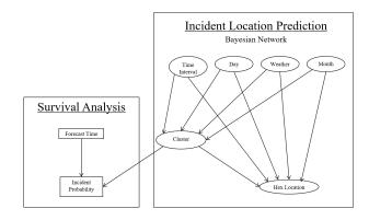
Fig. 3. Prediction Toolchain Model
