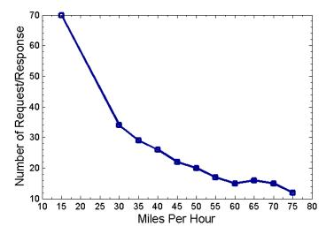
Figure 8: TCP-level packets delivered for different speeds
