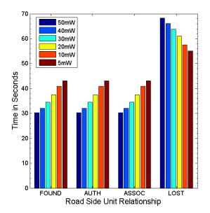
Figure 3: RSU relationship for single vehicle with varying radio power
