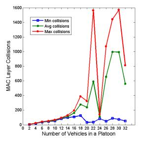
Figure 10: MAC-level collisions with increasing platoon size
