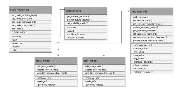
Fig. 2. Node Repository Class Diagram
