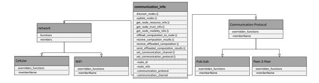
Fig. 5. communication info: class diagram
