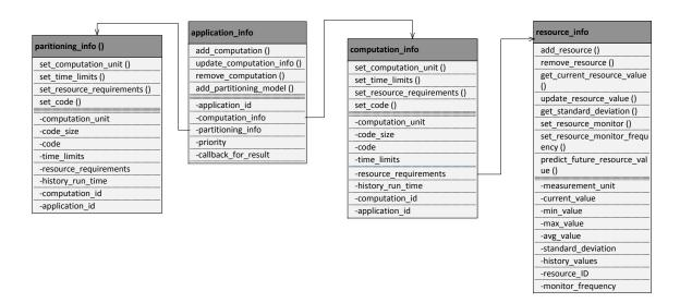
Fig. 4. Application Repository Class Diagram
