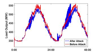
Fig. 10. Demand curve changes due to attacks aim for disturbing system operation
