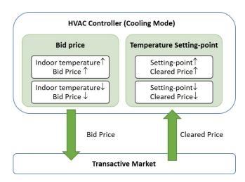
Fig. 4. Smart HVAC controller mechanism in cooling mode.
