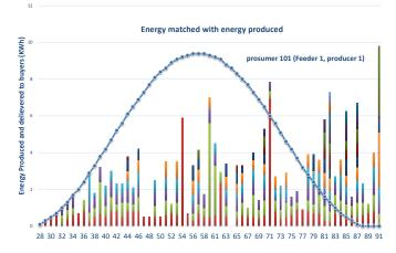
Fig. 7. Energy generated in each interval (blue line) and energy traded to a set of consumers in each interval (vertical bars) for the first prosumer of the first feeder. The stacked colors show the different consumers that were matched with the prosumer in each interval (note that the same color across multiple intervals does not necessarily mean the same consumer). When the energy traded exceeds the generation, the excess is drawn from the battery.
