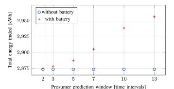
Fig. 6. Total amount of energy traded in the entire microgrid with and without batteries, for various prediction window lengths.
