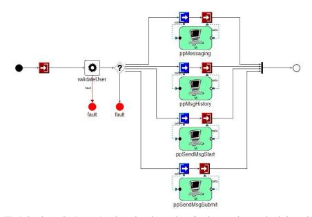
Fig 4. Service *ppSecInvocation* shows how invocation of various services can be tied together in a workflow. First the user gets authenticated by the *validateUser* task, which is a policy decision point implemented by the workflow. Assuming that the user gets successfully authenticated, the workflow decides which service to invoke based on user's input (such as a URL reference).
