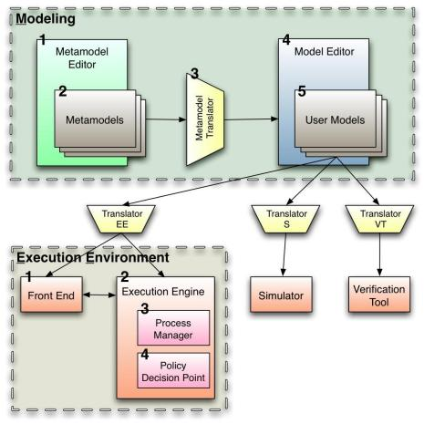
**Fig 1.** MICIS Architecture, where we facilitate the GME tool suite in the Modeling block to create a design environment for CIS. The models that are created in this design environment (the Model Editor) then can be translated as input for various analysis and execution engines.
