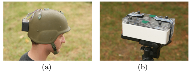
Figure 3: Sensor deployment prototypes mounted on kevlar helmets (a) and using plastic enclosures on tripods (b).
