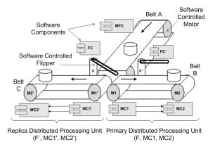
Figure 1: Reconfigurable Conveyor Belt CPS
