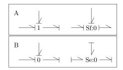
Fig. 1. Method of Implementing Hybrid Bond Graphs by Forcing Zero Effort/Flow in the Off Hybrid Junction
