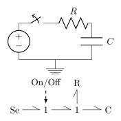
Fig. 3. Circuit Example and Unsimplified Bond Graph
