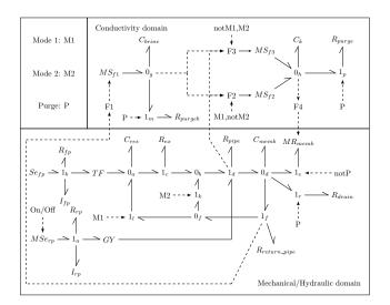
Fig. 14. Corrected Version of the RO System
