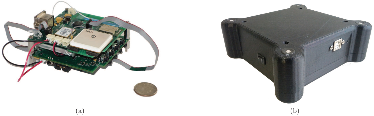
Figure 5: The prototype sensor node assembly (a) and packaging (b).
