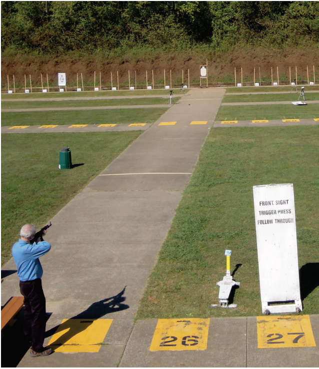
Figure 9: Shooting range with the four sensors on tripods in the distance. The green bucket in the foreground holds a repeater, as the TelosB we used for our remote user interface had trouble picking up the messages from the distant sensors.
