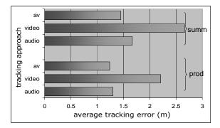
Fig. 7. Average tracking errors for all estimated tracks
