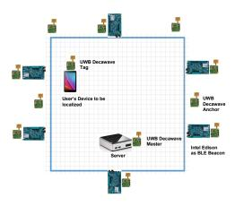
Fig. 2. Indoor localization experiment setup with 6 Intel Edison boards acting as BLE beacons;12 UWB Decawave sensors; centralized server for sensor processing and the android tablet whose position is to be localized.
