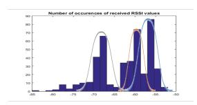
Fig. 1. A representative histogram of RSSI values received from a beacon node. The three peaks correspond to the mean RSSI value received on each of the three advertising channels, though the association between beacon messages and the corresponding channels is not available through the Android BLE API. By modeling the histogram as a mixture of three Gaussian kernels, the mean and variance of the RSSI values can be estimated on a per-channel basis.
