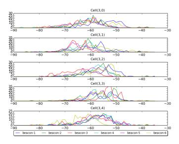
Fig. 3. Per-beacon RSSI histogram for adjacent grid cells in row 3.
